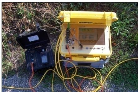
FIG. 03 – SISMOGRAFO UTILIZZATO MAE A6000S.
