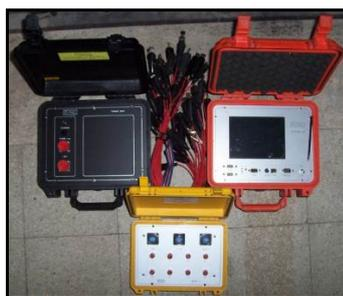
FIG.43 – GEORESISTIVIMETRO MAE A3000E, CON BOX DI ESPANSIONE E POWER BOX.
